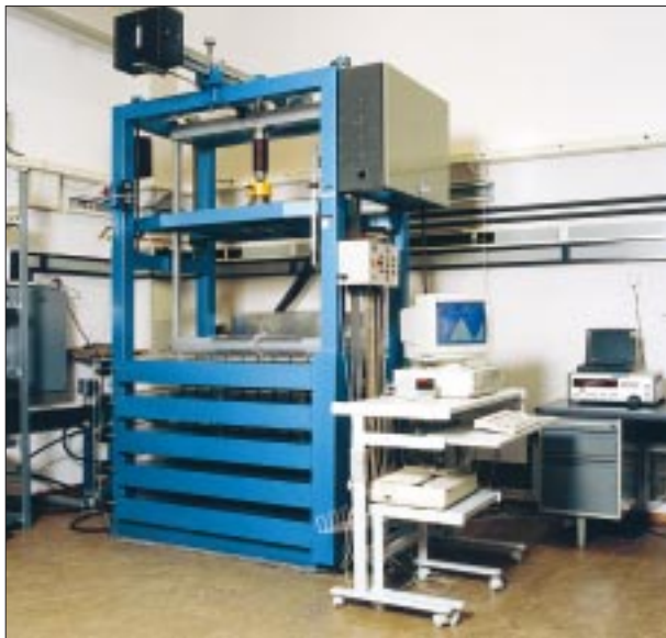
The 550 kg dead weight machine (see 2.1.2)
