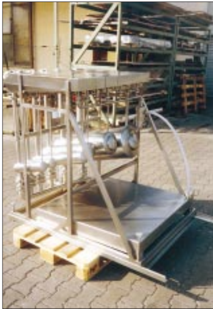
Fig. 5 Testing facility, normally mounted in a car for filling. Note the horizontally placed cylindrical provers made of stainless steel and the intermediate large storage tank lying on the ground.
