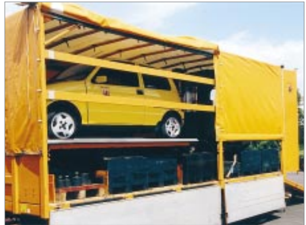
Fig. 4 Trailer: block weights beneath the passenger car and to the right and left of the forklift, which is standing on the loading area
