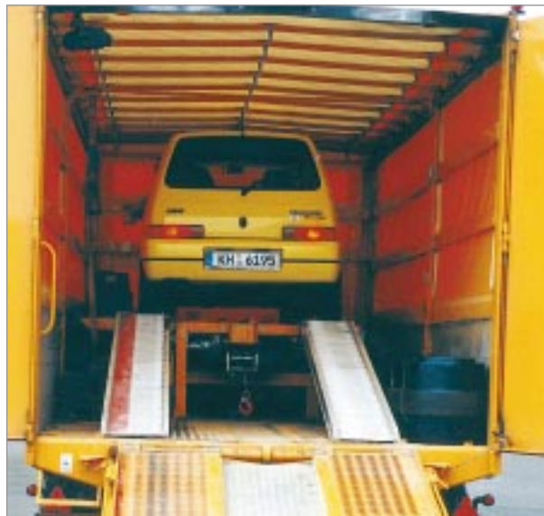
Fig. 10 Car in its final position on the trailer (beneath the car, winch for pulling up the forklift)
