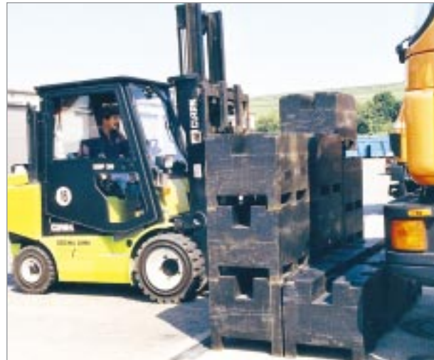
Fig. 7 Moving standard weights to special spots on the weighbridge
