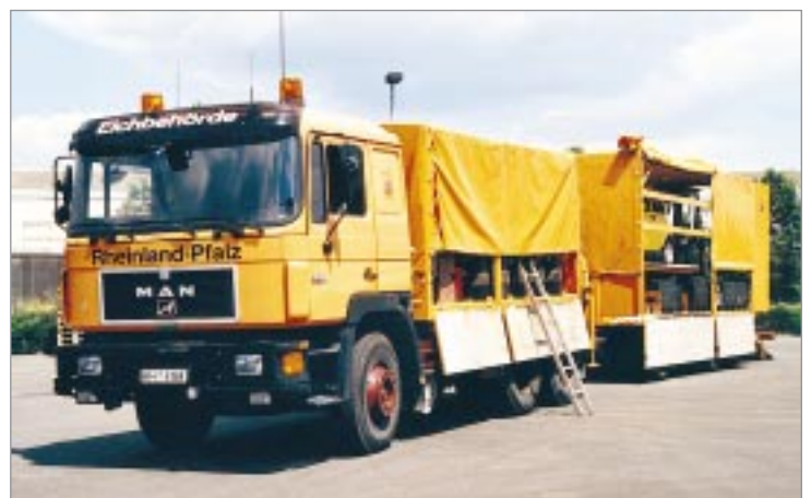
Fig. 1 Verification vehicle. On the tractor: 25 rolling weights (500 kg each); on the trailer: 15 t block weights, forklift and passenger car
