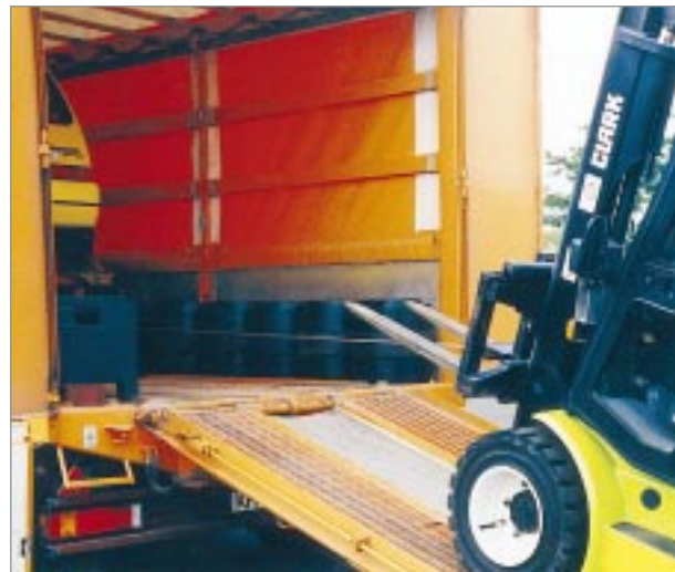
Fig. 8 Forklift pulled up by a winch
