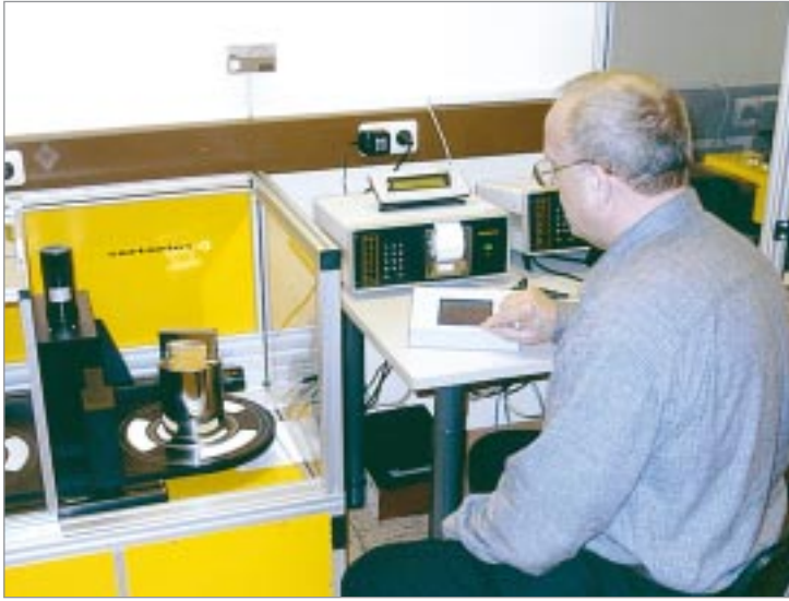
Automatic comparator weighing machine for the determination of weights up to 50 kg of accuracy class E 2 with scale controller
