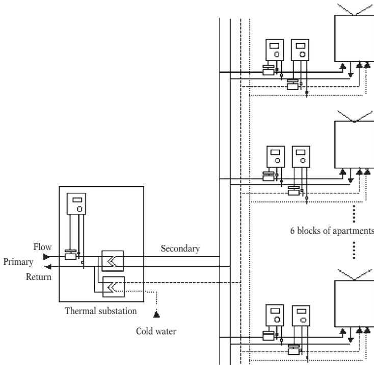
Fig. 3 Solution to meter heat and warm water at blocks of apartments
