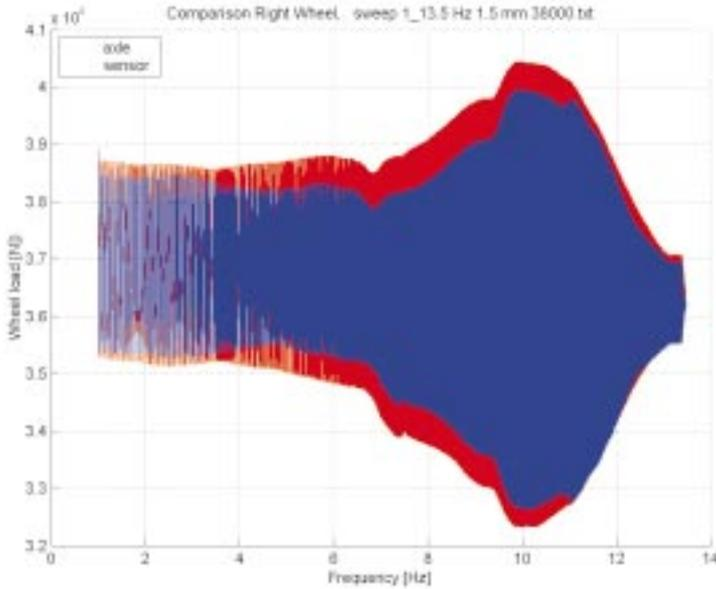
Figure 15 Right wheel, sinusoidal sinus sweep at 38 kN left and right wheel in phase
