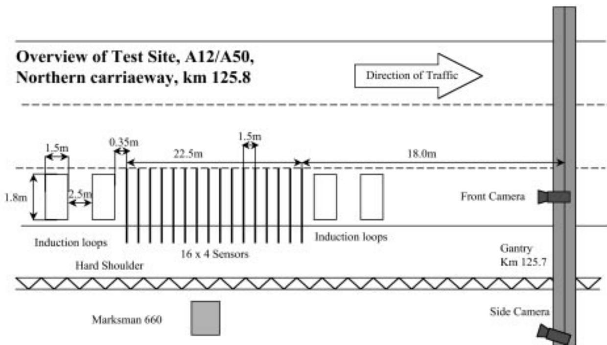
Figure 1 The WIM-Hand test system
