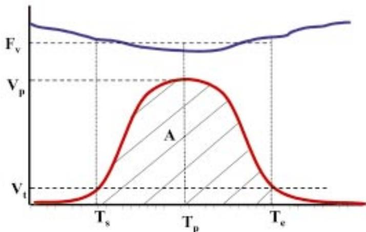
Figure 2 Example of signals measured by WIM-sensor (red) and vehicle (blue). Note: both lines in Figure 2 are examples to explain the measurement principle and not actual measurement signals.
