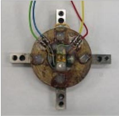
Figure 7 Set of mechanical strain amplifiers in a full bridge set-up
