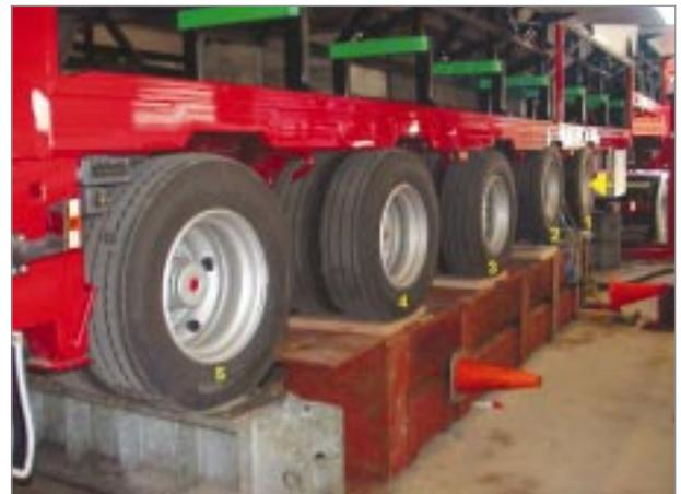
Figure 12 Levelled semi-trailer in the Lab for calibrating the measurement system
