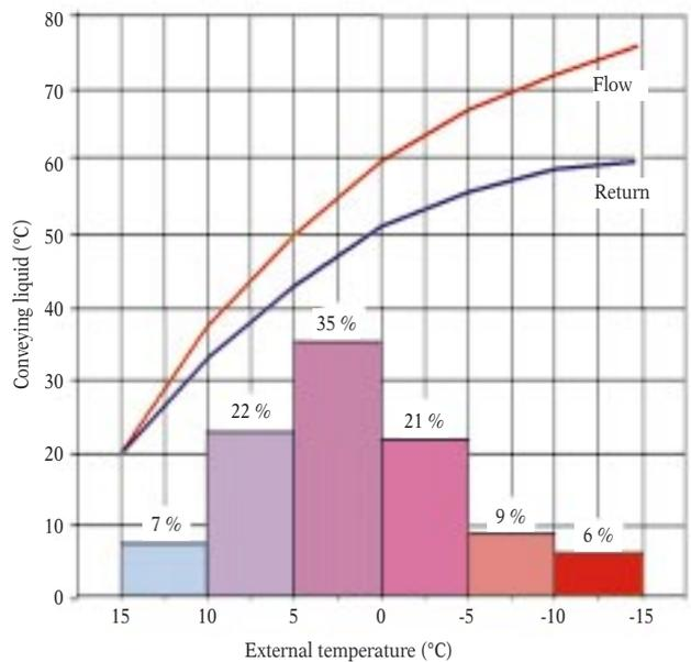
Fig. 4 Typical heat distribution chart
