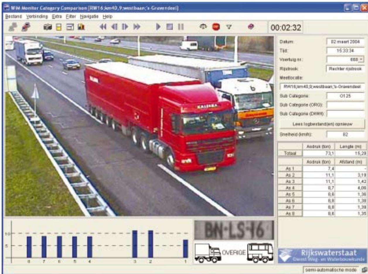
Figure 3 The instrumented vehicle in action
