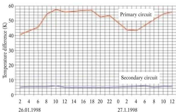
Fig. 5 Comparison between temperature differences in both primary and secondary circuits
