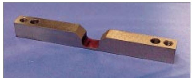
Figure 6 Mechanical stress/strain amplifier
