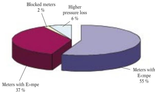
Fig. 2 Verification results of a sample from a batch of gas meters
