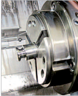
Figure 2: The weight blank is turned from a round steel bar
