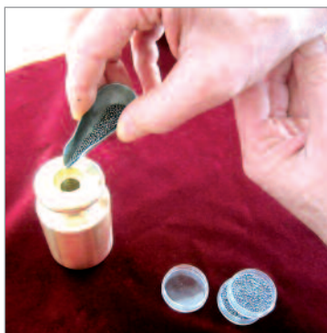
Figure 5: Filling the adjusting cavity
