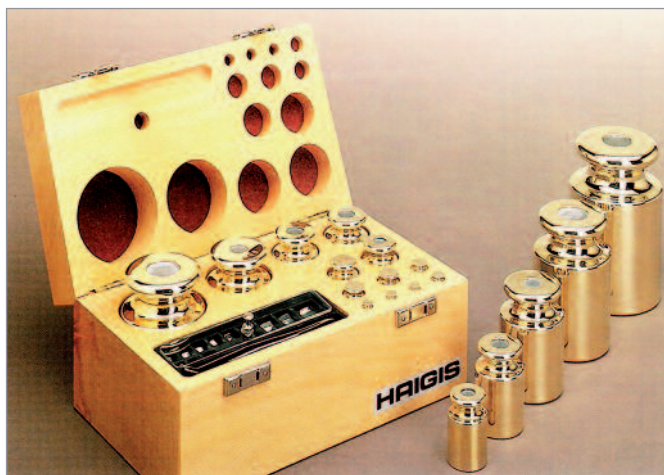
Figure 7: M_1 weight set in hardwood case
