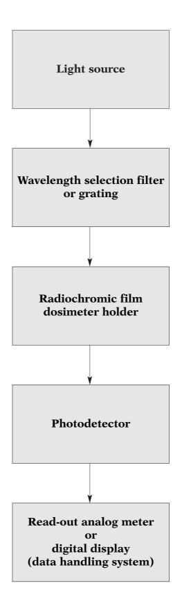
Fig. 1 Diagram of the read-out instrument used in a radiochromic film dosimetry system
